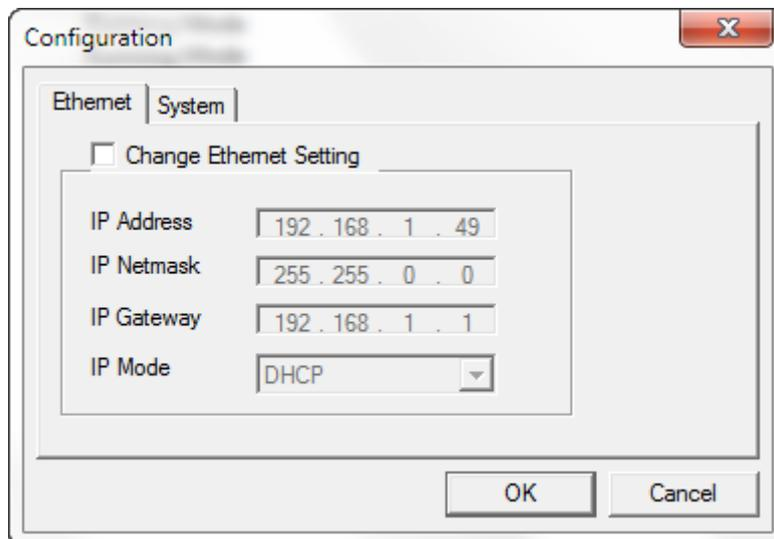
DHCP is on as default. You can change this to be static, by selecting 'Static IP' in the 'IP Mode'.
